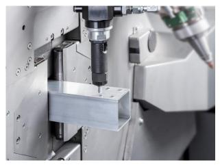
The fiber laser source allows wide maneuverability on different thicknesses and materials, ranging from 12 mm of mild steel to 4 mm of brass. 3D machining completes the picture of an extremely flexible system capable of spanning the most varied applications.
