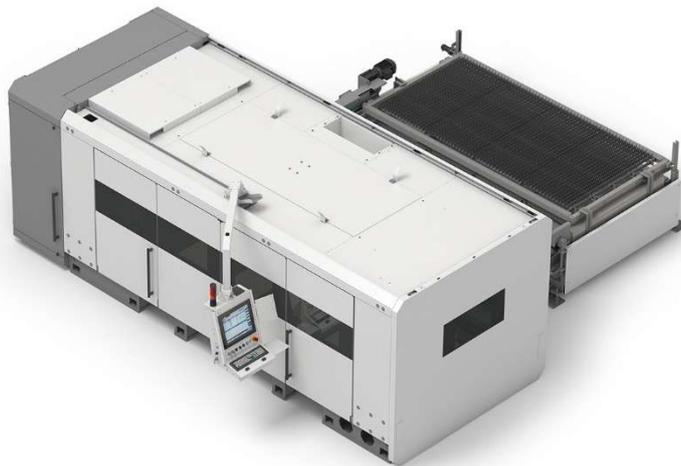
The LS5 can be equipped with Active Tools, a compiled suite of cutting-edge technical solutions to achieve the best results in less time regardless of the operator's experience: Active Piercing for increased cutting performance on thicker material, Active Cool for improving the workpiece cutting quality using water cooling, Active Camera for helping the operator to make the most of the material by managing the nesting with a simple drag&drop method on the machine interface screen, and
